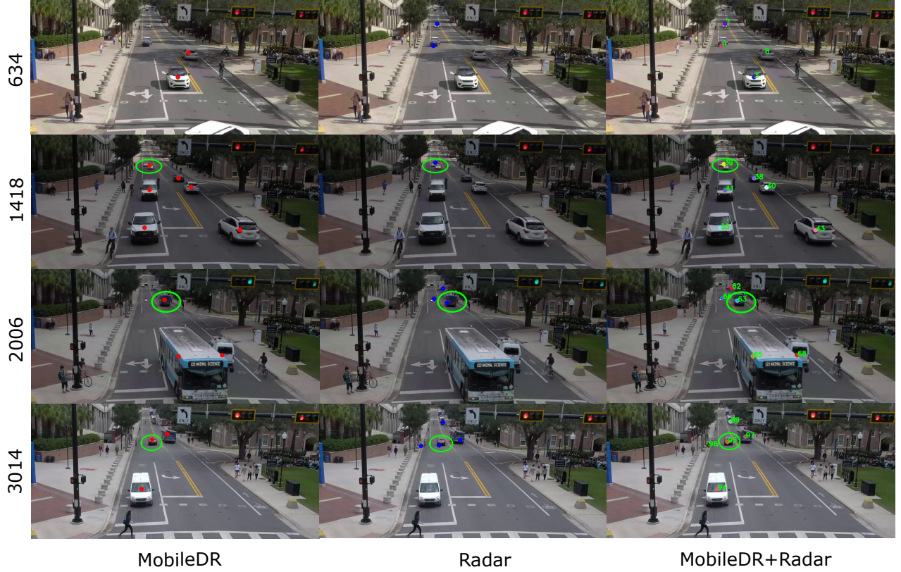
Figure 6: Tracking outputs for Easy sequence (frames 634, 1418) and Hard sequence (frames 2006, 3014). We highlight tracks that overlapped between sensors and were subsequently matched and fused. We show the IDs of the fused tracklets.
